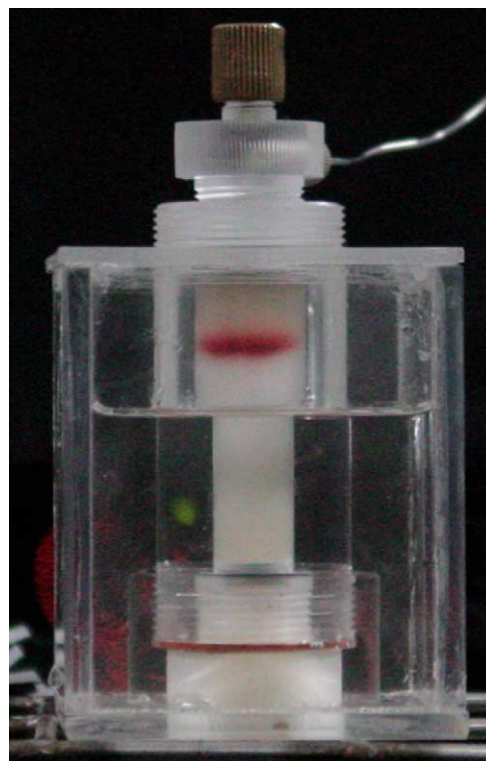
Fig. 2. Photograph illustrating the cylindrical lens effect using the reservoir half filled with glycerol.
